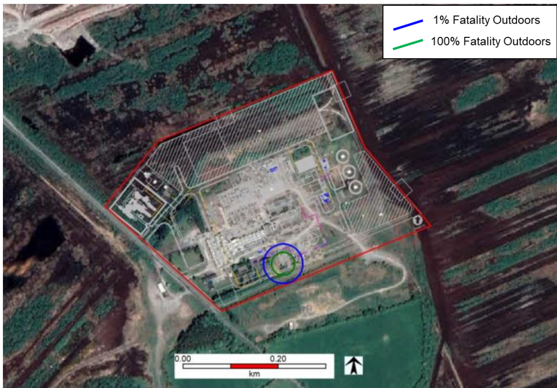
Figure 33 LPG Tank Rupture and Fireball: Outdoor Lethality Contours
