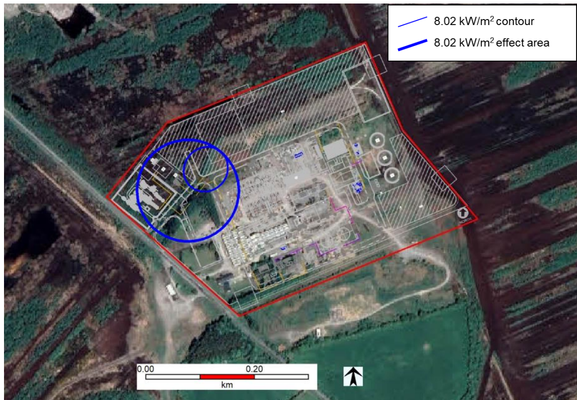
Figure 12 Horizontal Pipeline Leak and Jet Fire: Thermal Radiation Contours Corresponding to 1% Mortality Outdoors
