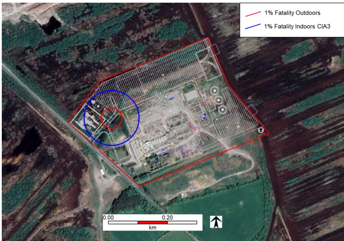
Figure 19 Pipeline Leak (Horizontal) and VCE: 1% Fatality Outdoors and 1% Fatality Indoors CIA. 3 Contours
