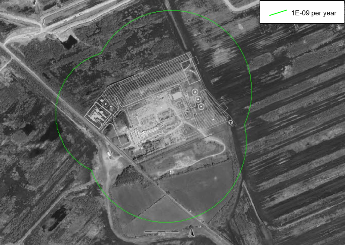
Figure 114 Individual Risk Contour, to Persons Indoors CIA Cat. 3, Corresponding to 1E-09 per year (Consultation Distance)
