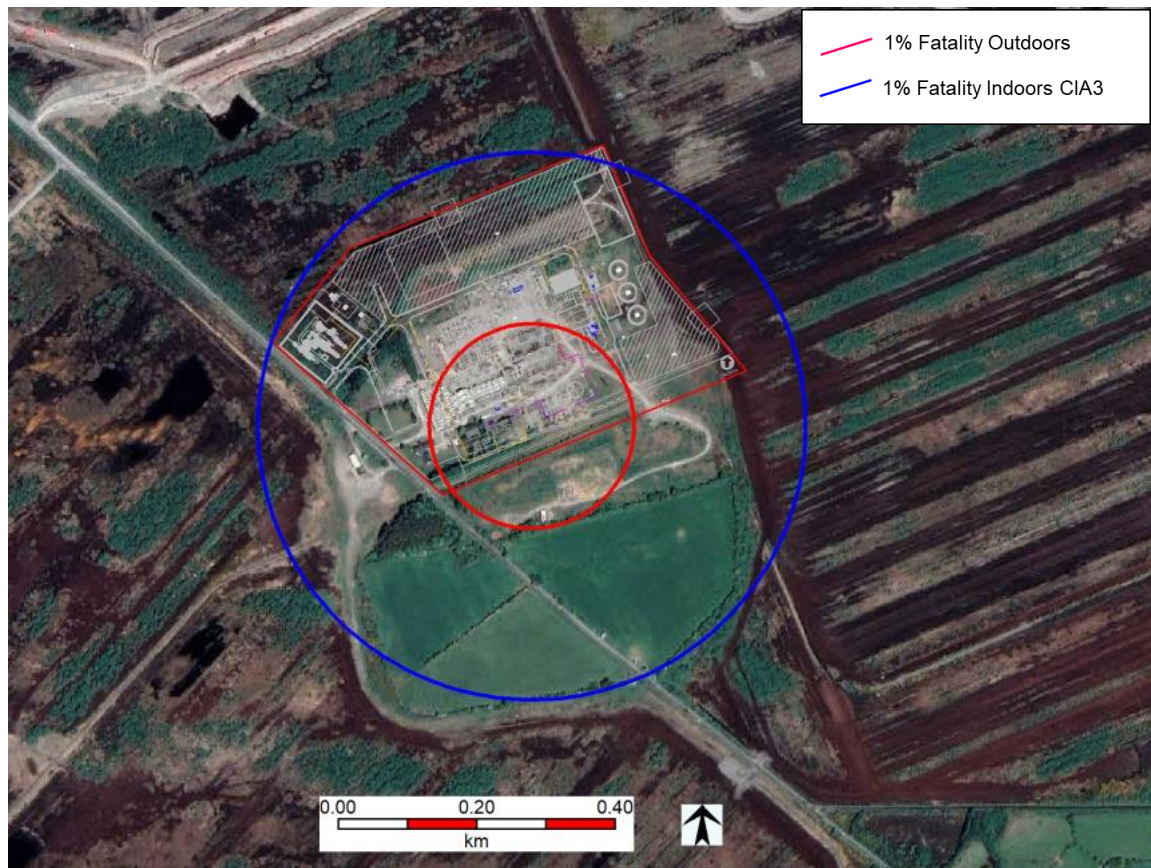
Figure 67 LPG Tanker Rupture and VCE: 1% Fatality Outdoors and 1% Fatality Indoors Overpressure Contours
