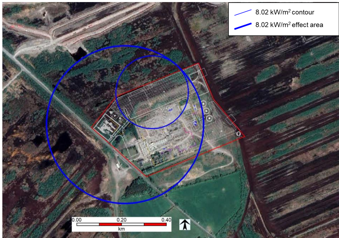
Figure 11 Horizontal Pipeline Rupture and Jet Fire: Thermal Radiation Contours Corresponding to 1% Mortality Outdoors
