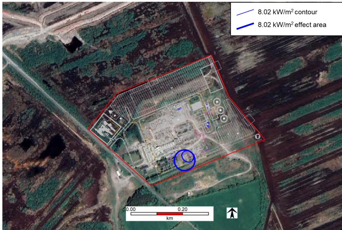
Figure 46 LPG Tank Horizontal 10mm Leak Over 30 Minutes and Jet Fire: 1% Fatality Outdoors Contour
