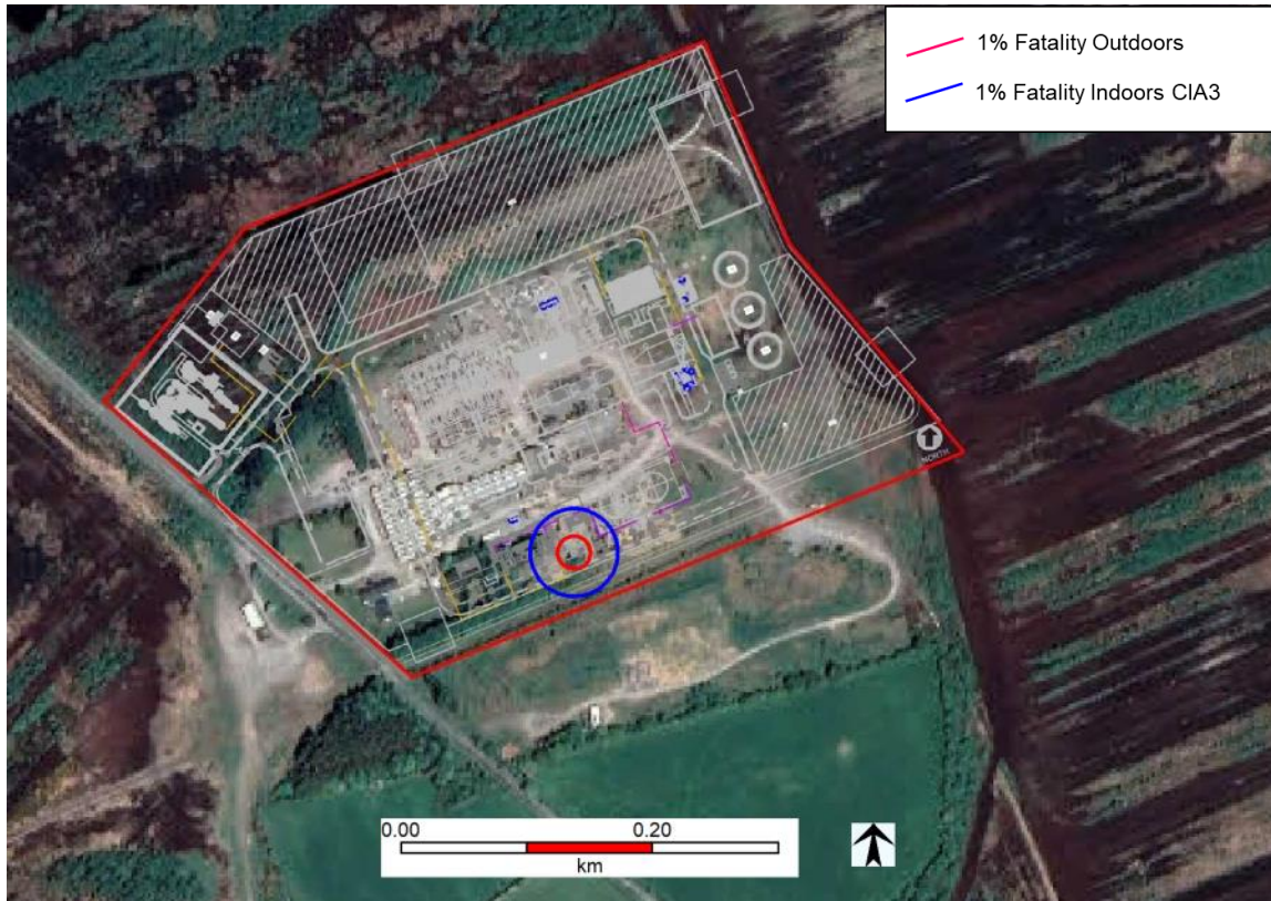
Figure 49 LPG Tank Horizontal Tank Leak and VCE: 1% Outdoors Fatality Contour and 1% Fatality Indoors CIA Cat. 3
