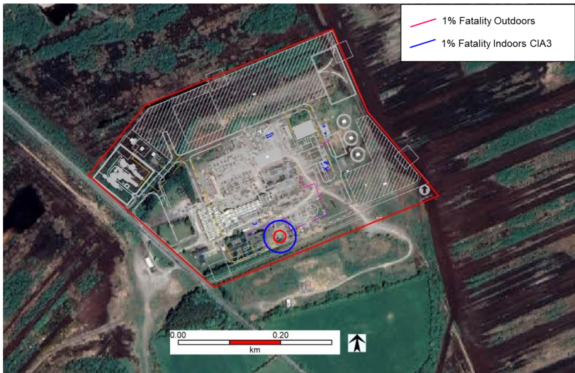
Figure 84 LPG Tanker 10mm Hose Leak and VCE: 1% Fatality Outdoors and 1% Fatality Indoors CIA Cat. 3 Overpressure Contours
