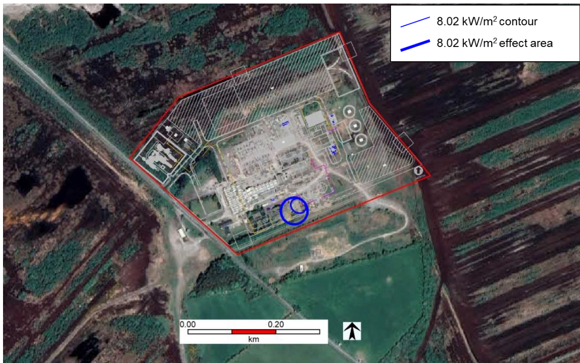
Figure 40 LPG Tank Horizontal Leak Over 10 Minutes and Jet Fire: 1% Fatality Outdoors Contour
