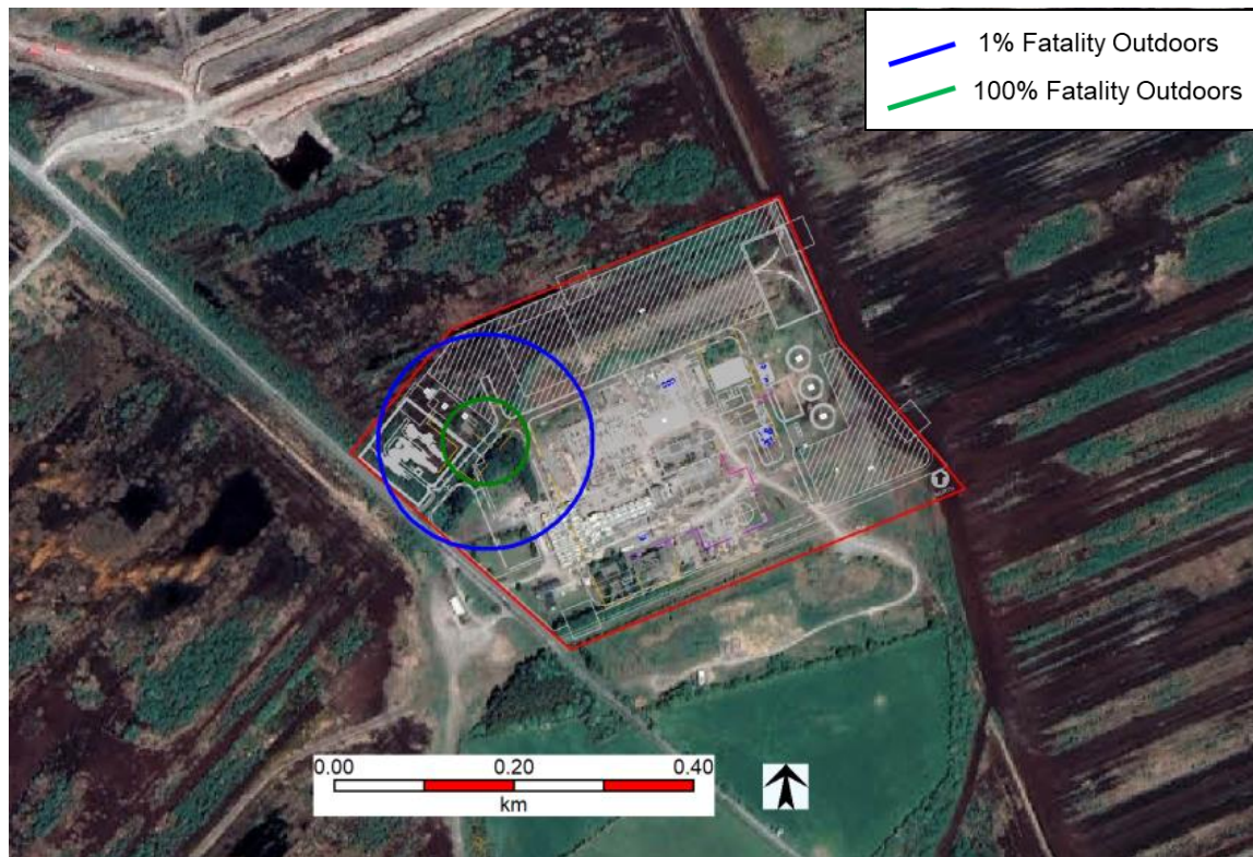
Figure 16 Pipeline Rupture and Fireball: Outdoor Lethality Contours
