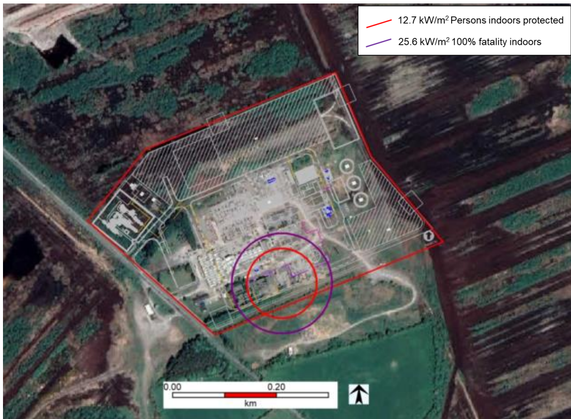
Figure 34 LPG Tank Rupture and Fireball: Indoor Lethality Contours
