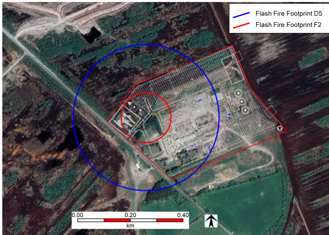
Figure 24 Pipeline Rupture (Horizontal): Flash Fire Footprint
