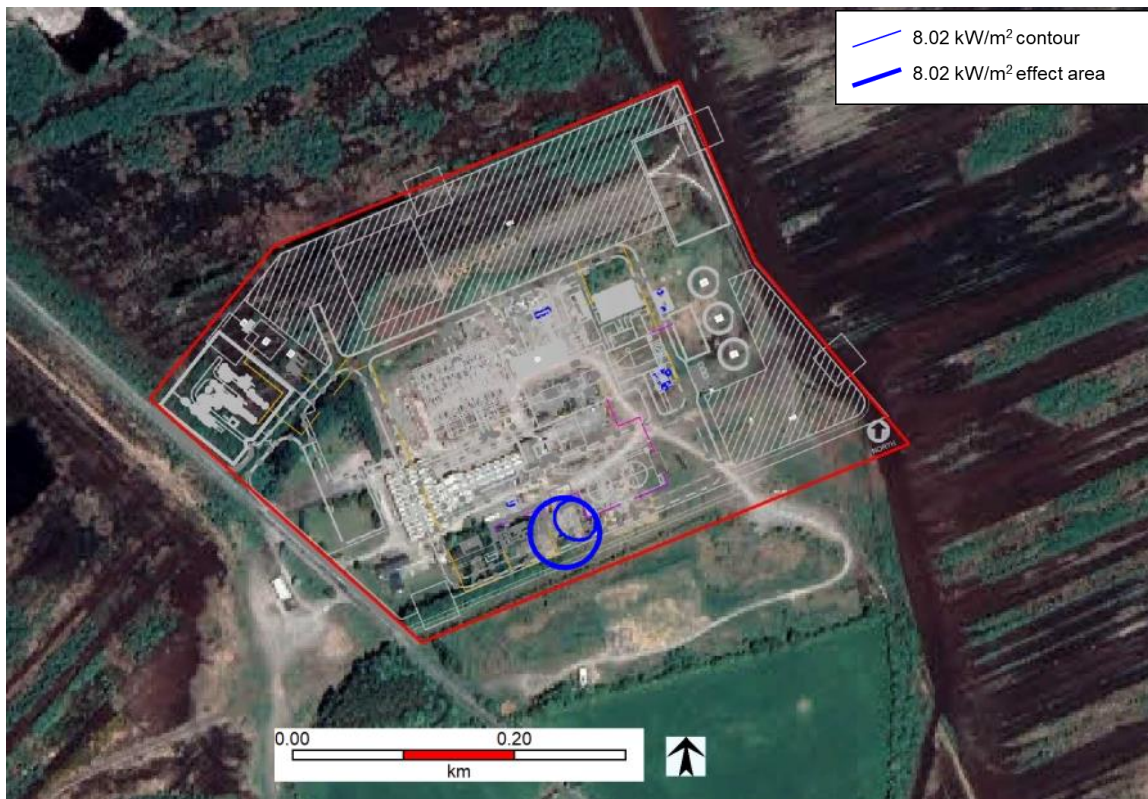
Figure 81 LPG Tanker 10mm Hose Horizontal Release and Jet Fire: 1% Fatality Outdoors Contour
