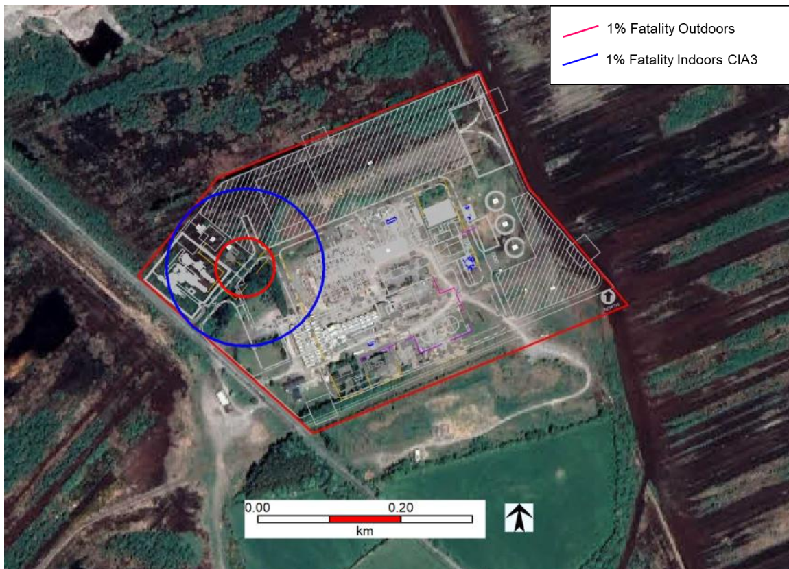
Figure 18 Pipeline Rupture (Horizontal) and VCE: 1% Fatality Outdoors and 1% Fatality Indoors CIA. 3 Contours
