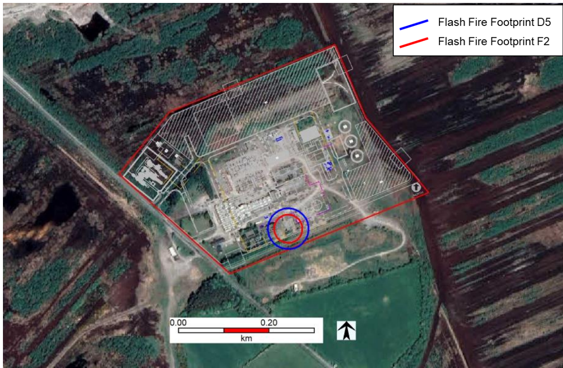
Figure 37 LPG Tank Rupture and Flash Fire: Flash Fire Envelope
